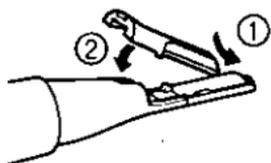
2. Slide the blade lock in the direction indicated below.
